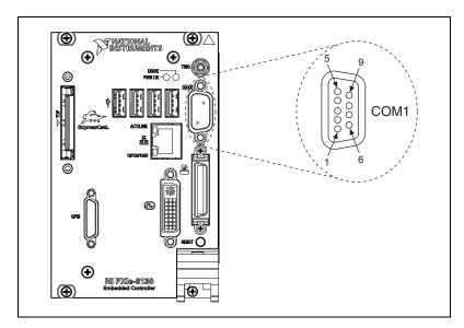
Figure 3-3. COM1 Connector Location and Pinout
